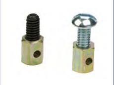
The inner cable goes through the hole on the body of the wire stop and the set screw gets tightened into place. They are compatible with both solid and stranded wire. Wire stops are designed to be field installed on one side of a pull control.
