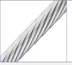
Typical stainless steel cable railing is 1 × 19 construction. 1 × 19 stainless has minimal stretch, ideal for tensioning. It appears clean and shiny in comparison to other constructions and materials.
