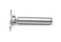
The outside diameter of a classic turnbuckle body tapers to a smaller diameter at the ends. In a Decko, there is no taper, which means that the turnbuckle body is one outside diameter for the body length. This turnbuckle is commonly selected based on style preference. Deck toggle pictured to the left. Toggle jaw, ball, and button also available
