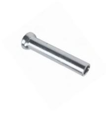
It's popular to have a non-tensioning (fixed) fitting at one end of a cable railing. Fixed fittings are smaller and more economical than their turnbuckle counterparts. As a general rule of thumb, if the assembly is less than 50 feet long and is not making any bends, then a fixed fitting at one end would be an appropriate option.
