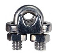
A wire rope clip is comprised of a u-bolt with a saddle and hex nuts. It is most commonly used to form loops. Because you only need a wrench to tighten the nuts, the wire rope clip is ideal for field installations. For diameters 7/16" and below, a minimum of 2 wire rope clips is recommended for a loop. For diameters 1/2" - 5/8", a minimum of 3 wire rope clips is recommended for a loop. For diameters 3/4" - 7/8", a minimum of 4 wire rope clips is recommended for a loop.
