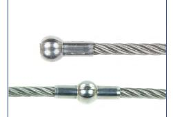
Typically installed at the end of a wire rope assembly, single shank balls may also be installed at an intermediate point. Single shank balls are widely available in stainless steel per MS20664. In some sizes, Lexco also carries single shank balls in zinc-plated steel. Single shank balls are designed to be rotary-swaged with tool and die (not recommended to handcrimp).
