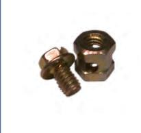
The threaded stud has a blind hole on one side where a wire rope is inserted, and external thread on the other. The name "threaded plug" is typical when the crimp area and cable hole within are both short. Overall, the entire length of a threaded plug is smaller than its counterparts in this product line. "Threaded terminal" is a term that's used when the threaded stud is for an architectural cable railing or marine cable application. "Swage stud" is an alias for a threaded stud.
