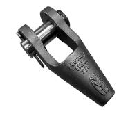
A spelter socket is attached to the end of a wire rope by either resin compound or poured zinc. Spelter sockets come in different styles, such as closed eye and open clevis. Installation of spelter sockets is recommended to be performed in a controlled environment, such as a wire rope rigging shop.
