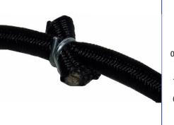
A solid steel wire is crimped onto the cord. Usually the cord is folded back before crimping to create additional surface area for the termination. Single crimp means one revolution of wire is crimped around the cord, while double crimp means
