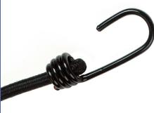
Bungee hooks are the most common bungee cord end fittings. The typical hook is metal with a black PVC cover, but Lexco can also supply hooks made from steel and stainless steel. The hook can be attached to the bungee cord in a few different ways: a knot or a wire crimp (also known as a hog ring) can be formed to retain it, or a crimped button stop or similar ferrule can be used to retain the hook in some designs.
