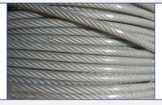
The nylon coating is a jacket. With nylon, there are different resin types within the nylon family. The majority of nylon coatings fall under the nylon 6 family. When higher performance is required, we coat in the nylon 11 family since nylon 11 can handle higher cycling applications with more rigorous friction. MIL-DTL-83420 Type 2 Utilizes a nylon 11 jacket.
